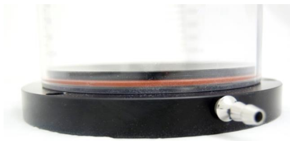
Canister and tube CORRECTLY attached
