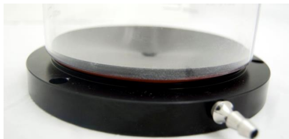
Canister and tube INCORRECTLY attached
